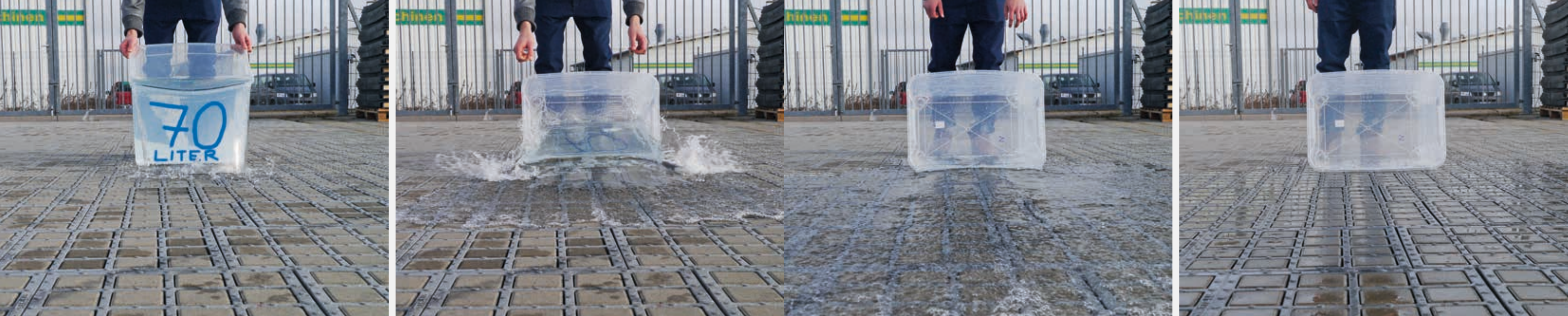
A practical test proves: 70 litres of water seep away in less than one minute on an area of about 6 m 2
